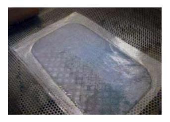
Sections of Spaceloft insulation were laminated for easy insertion into the sleeping system. A fast, efficient lamination process is being developed for mass production.
