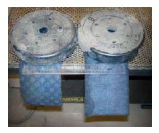
Spaceloft insulation was diamond-scored, giving it the complete flexibility needed for sleeping system use. Scoring had minimal effect on the thermal conductivity of the insulation.
